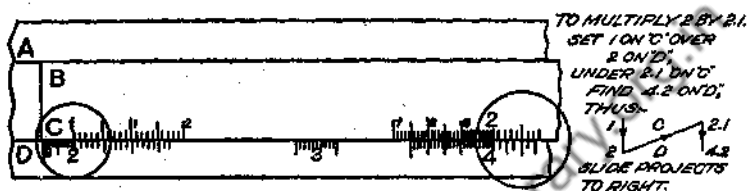
FIG. 4(a)—Multiplying Numbers on the Slide Rule
